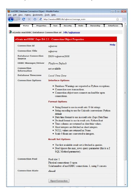
This shows the connection object details as well as the currently active connection options and the state of the connection pool associated with this connection object.
