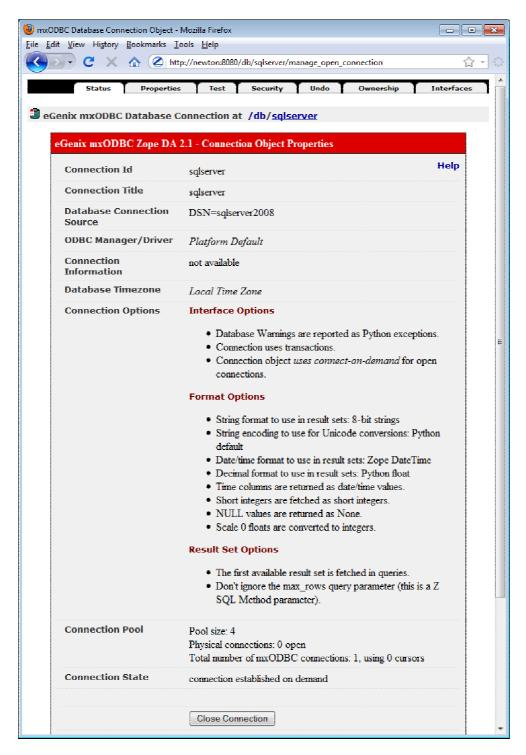
Note that under heavy load, the physical connections may not be freed immediately. This is due to the multi-threaded nature of Zope. Opening and closing the connection again usually helps in these rare cases.
