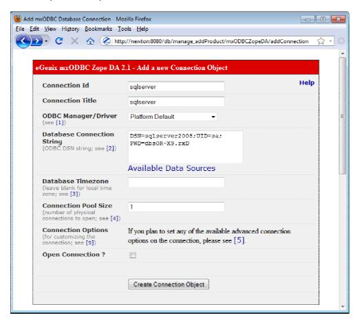
Hitting the Create Connection Object button will create the mxODBC Zope DA connection object, possibly trying to open the physical connections provided that you have chosen to create an open connection.
