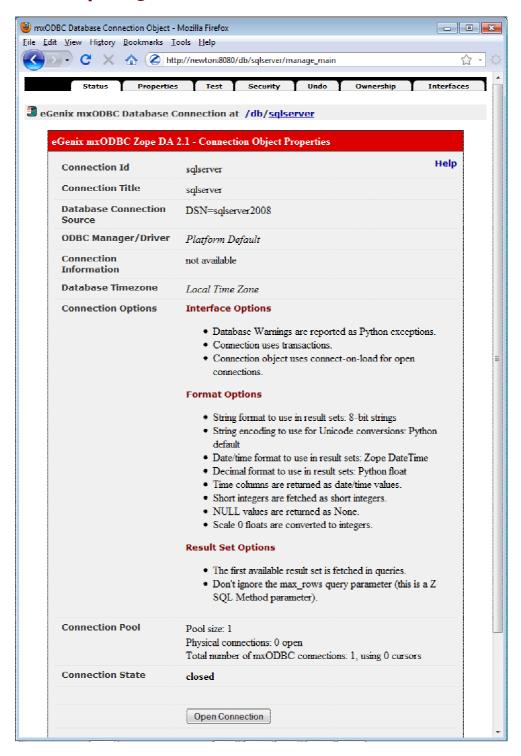
To open the connection, simply press the button Open Connection. Note that the button is only visible in case the connection is closed.
