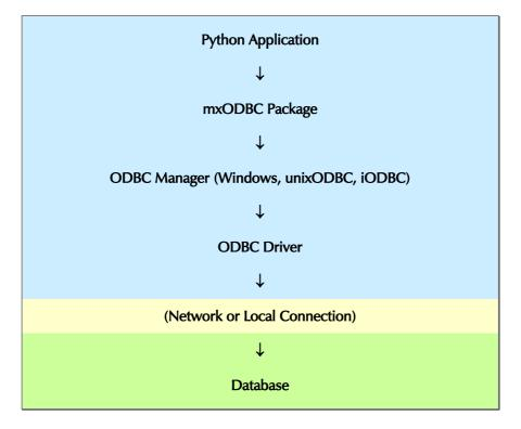
The upper blue part in the diagram executes within the process of the Python application. The green part usually runs in a separate process and possibly also on a different machine.
