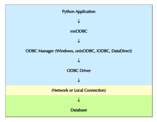
The upper blue part in the diagram executes within the process of the Python application. The green part usually runs in a separate process and possibly also on a different machine.
