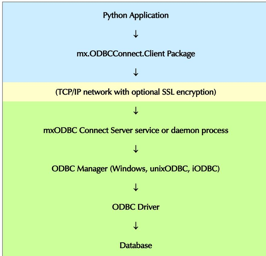
The upper blue part in the diagram executes within the process of the Python application. The green part usually runs in a separate process and usually also on a different machine.
